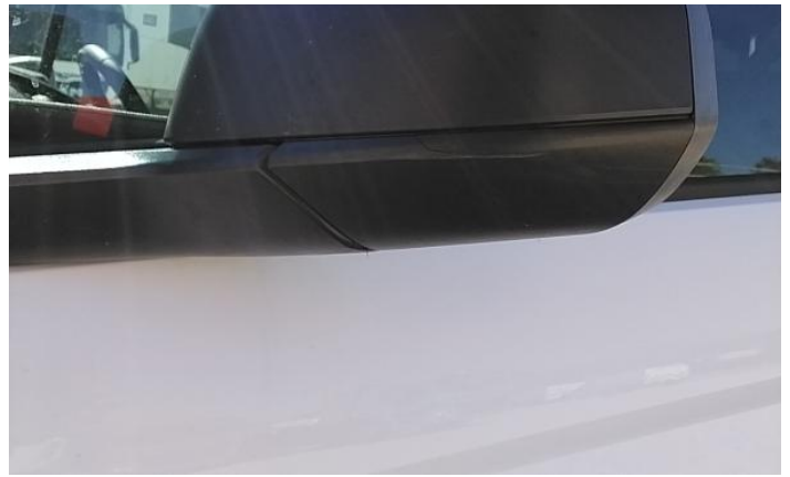
4: Wing nsf Dented Between 10mm + 30mm
