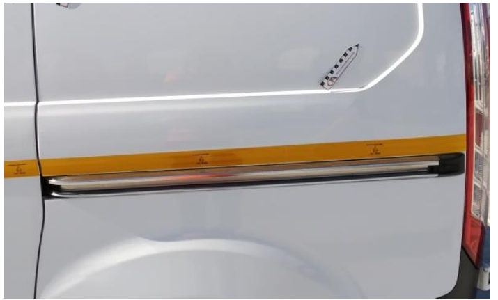
4: Door nsf Scratched Over 25mm Thru Paint
