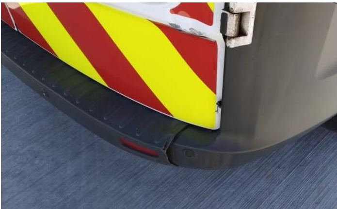
5: Qtr Panel nsr Dented With Paint Damage
